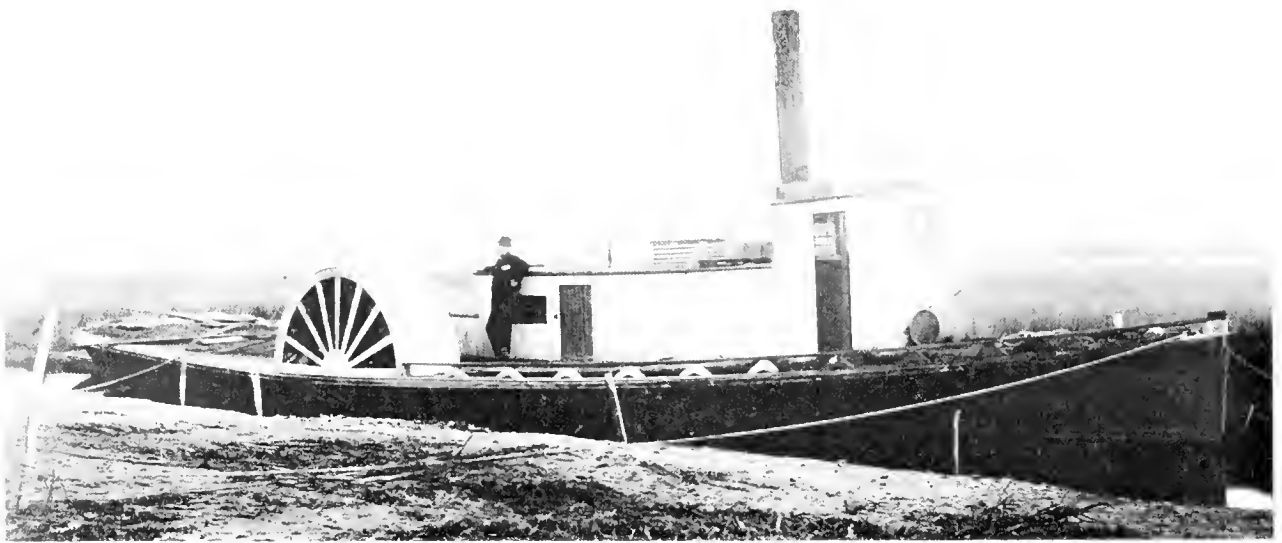
PADDLE-WHEEL FISHING STEAMER BUILT IN 1885 FOR SERVICE ON THE NORTH CAROLINA SOUNDS, the Camille . A model of this steamer, USNM 76236, is in the Watercraft Collection. (Smithsonian photo 34648-a.)
